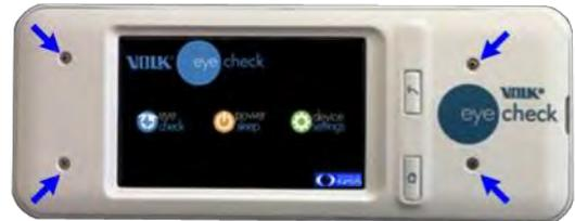
2. Gently pry the back cover away from the front of the Eye Check device, starting at the groove on the right-hand end of the case.
