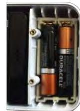
4. Replace the back cover by snapping it in to position all around the edges. Finish by replacing the four screws saved from step 1.
