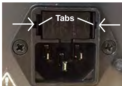
Figure MM-01 Fuse Holder Tabs
