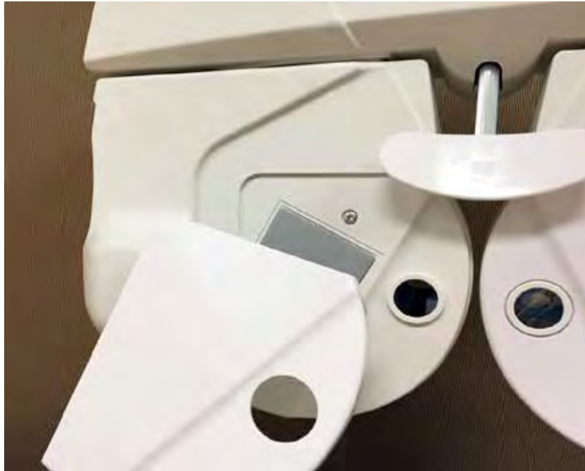
Figure IS-13 Install Face Shield
