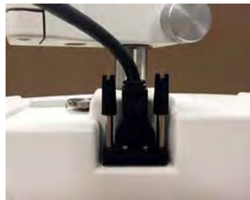
Figure IS-09 Cable Installed
