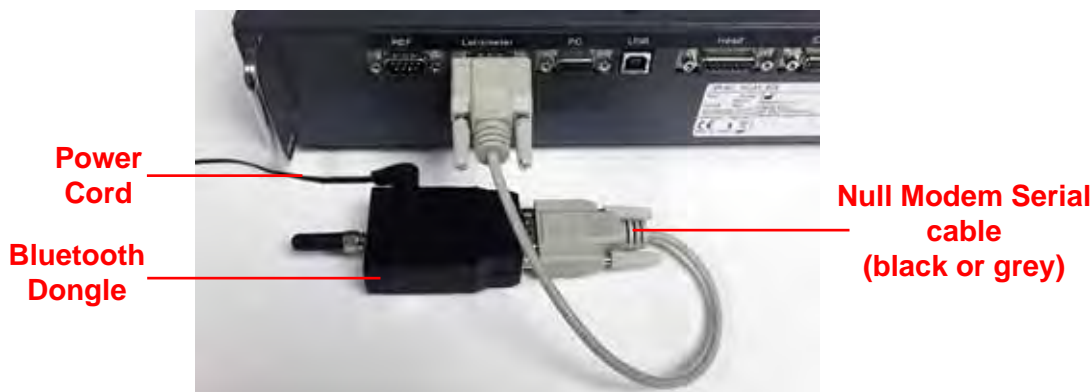
Figure IS-16 Bluetooth Dongle to Relay Box Assembly
