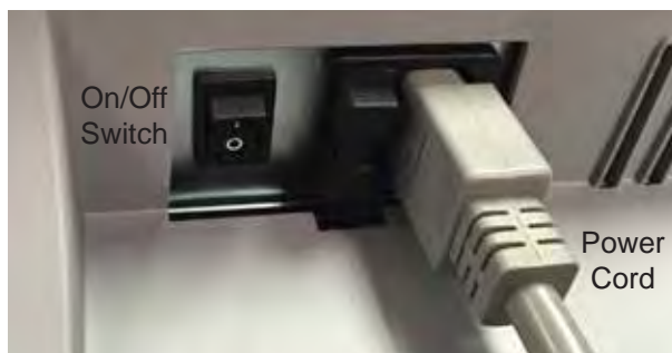
Figure SU-18 Power Cord and On/Off Switch
