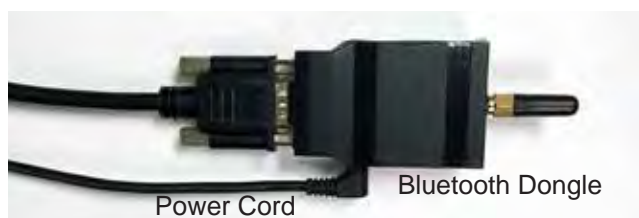
Figure SU-23 Connect Dongle to Power
