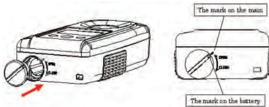
2. Align small mark found on the battery cover with mark found on the instrument body and insert cover as shown above.
