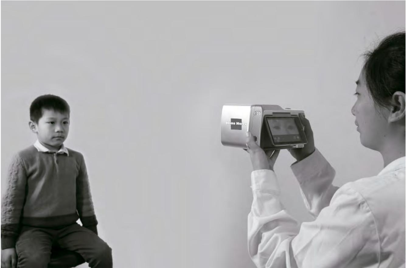
The Cell vision screener HVS001 is a portable diagnostic device designed for clinicians to quickly detect vision abnormalities on patients from 6-month old to adults. Cell can screen both eyes at once from a distance of 1 meter. Once the pupils are in focus, the device will start to calculate automatically and deliver results within 1 second. The touch screen allows users to operate conveniently like using a smart phone.
