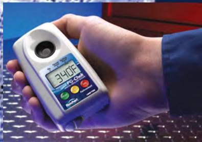
**Fire Sprinkler Systems:** The Reichert PG-Chek can be used to measure the concentration of antifreeze formulation in wet fire sprinkler systems. An NFPA-compliant antifreeze should not exceed 38% Propylene Glycol concentration (National Fire Protection Association).
