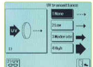
The measured data can be saved and the UV transmittance of multiple lenses can be compared.
