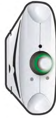
Incorrect alignment of the tonometer. Readjust so that you see only the front of the tonometer and the green light symmetrically in the center of your view.
