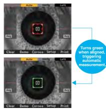
Smooth and accurate alignment function. Once aligned, air pulse and measurement commence automatically.
