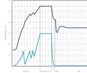
\*Three air removal purges. Electronic bellows purge air from chamber three times prior to sterilization for efficient air removal.
