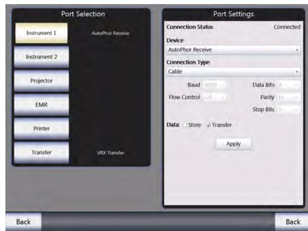
**Figure IS-20, Port Setting for Receiving Data from the previous VRx in a daisy chain**
