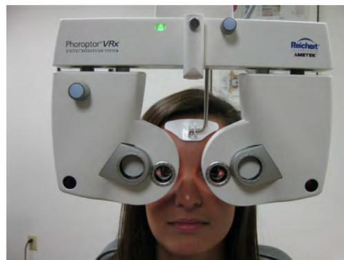
**Figure IU-03, Adjust Phoropter Head**
