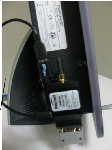
**Figure IS-15, ClearChart Bluetooth Dongle Mount**
