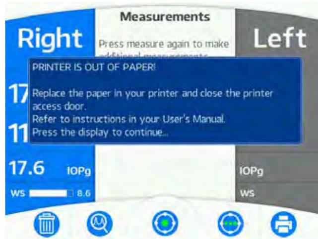
**Note:** If the printer paper runs out before printing all the measurement data, the data will be stored. Once the printer paper is replaced, a complete print out of all measurement data will start.
