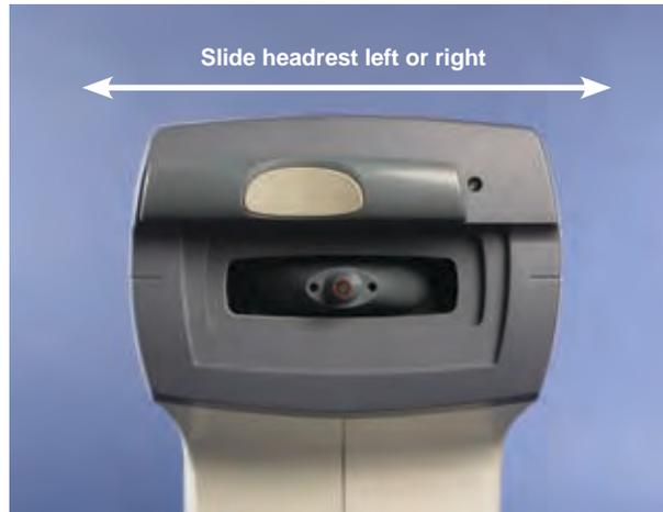
The Ocular Response Analyzer G3 features a left/right sliding forehead rest that enables the instrument to determine which eye is being measured. It must be positioned completely to one side or to the other in order to take a measurement. Position the forehead rest to the desired position before beginning the measurement process.
