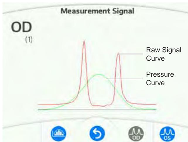
The measurement signals based on the best waveform score obtained can be seen by tapping the corresponding icon, either OD or OS. This signal displays the Applanation Curve (red line) and the Pressure Curve (green line).
