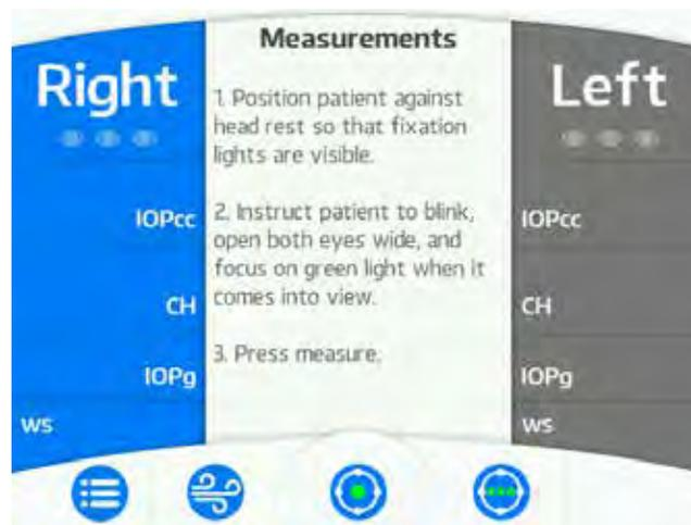
**Note:** To ensure fast and accurate results operators should instruct the patient to blink a few times and hold both eyes open immediately before measurement. Remind the patient to look directly at the green light and hold steady.
