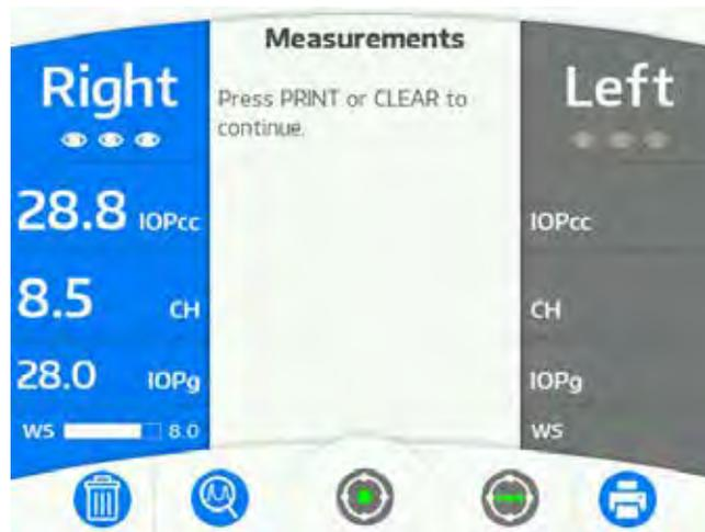
The unit will go into sleep mode after the specified amount of time selected in the Setup Menu. When the unit comes out of sleep mode, any measurements that were not cleared out prior to sleep mode will appear on the screen, but the measurement buttons will be disabled in order to prevent accidentally combining data from two different patients.
