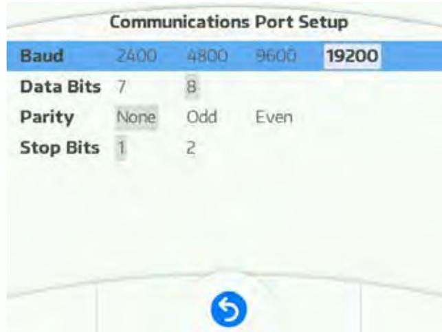
The Ocular Response Analyzer G3 can transfer data to an external device, such as a computer, through the RS232C port.
