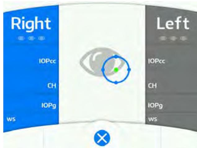
During the alignment and measurement process, the Operator Display will show the position of the airtube with respect to the center of the patient's cornea. As the positioning system aligns to the apex of the eye, the measuring icon will move to the middle of the screen and align over the center of the eye graphic. Once the positioning system is aligned the air puff(s) is delivered to the eye and the measurement results are automatically displayed.
