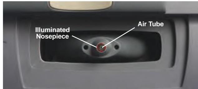
A properly positioned patient will easily see the fixation cues. The fixation target is a green light, located inside the air tube, surrounded by a ring of red lights. In order to take a measurement, patients must be fixating on the green light. If a patient is able to see any of the lights (red or green) then patient position is adequate. If any red lights can be seen, the automatic alignment system will bring the green fixation target into view. The measurement will be made automatically.
