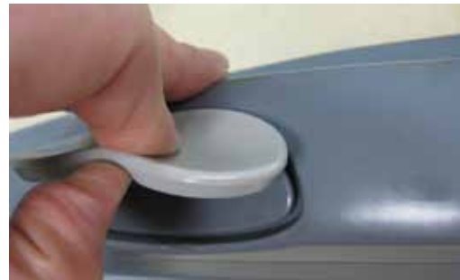
Figure CL-3. Remove Forehead Rest Pad
