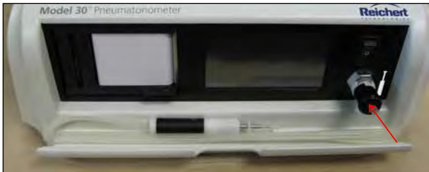
Figure 1-10, Probe Connection
