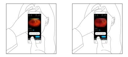
The correct imaging distance is reached when the retina completely fills the imaging window. Do not be afraid to gently push the device closer to the patient - the eye cup is flexible and the device will not touch the patient's eye. If auto-focus is enabled, tap anywhere on the screen to focus, except for a button. A green box will appear when the retina is in focus.
