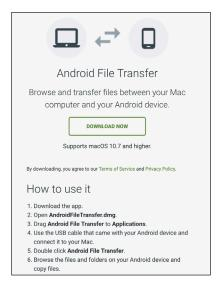
Connect the device via USB-C cable to a Mac. Pull down from the top of the phone homepage to view the Android system options and select **Tap for more options**. Make sure to select the File Transfer option on this screen to connect the VistaView to a PC.
