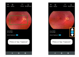
To capture an image, ensure that the full field-of-view is illuminated with no dark spots, reflections, or shaded regions appearing toward the boundaries during preview. Press the **Capture** button on screen. The device will flash and capture an image. If **Voice Capture** is on, wait for the green box to appear if using auto focus then take an image by saying the word "Capture".
