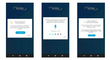
For best results when using the **Voice Capture** feature on the VistaView, the user can train the device to recognize their voice and pronunciation of the word "Capture". Press **Continue** to begin training. When you are ready, tap the microphone icon and repeat the word "Capture" five (5) times. The screen will update after each successful training attempt. You can also repeat this training at any time by following the steps under Voice Capture Settings in the next section of this IFU.
