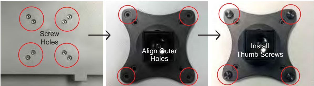
Figure SU-10 Align Holes and Attach Mount
