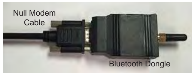
Figure SU-18 Connect Dongle to Cable
