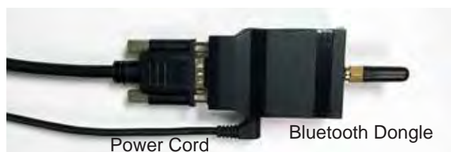
Figure SU-20 Connect Dongle to Power
