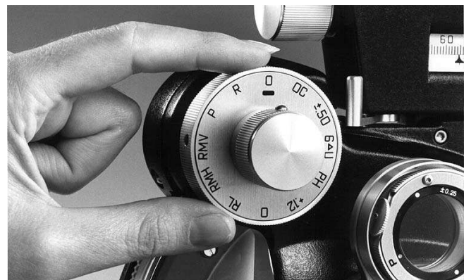
Figure TM-4 Rotating Strong Sphere Control (Surrounds Auxiliary Lens Scale)
