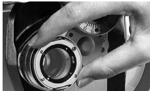
Figure JC-6 Rotate Cross Cylinder
