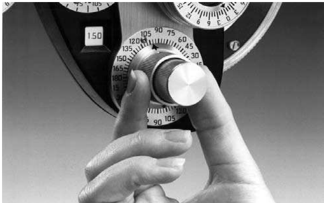
Figure TM-6 Turning Cylinder Axis Knob
