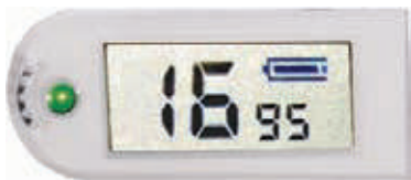
Figure 4. Closeup of TONO-PEN AVIA VET Tonometer LCD showing an IOP measurement of 16 and statistical confidence indicator of 95
