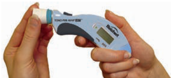
Figure 3. TONO-PEN AVIA VET Tonometer Preparation
