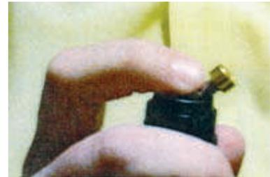
When using the eyecup simply attach the transducer (screw clockwise) onto the probe scan head finger-tight and it is ready.
