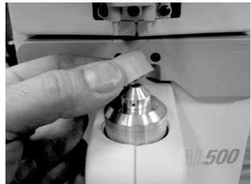
Figure 18. Contact Lens Holder
