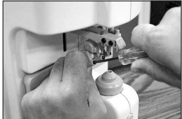
Figure 22. Marking Pen Removal
