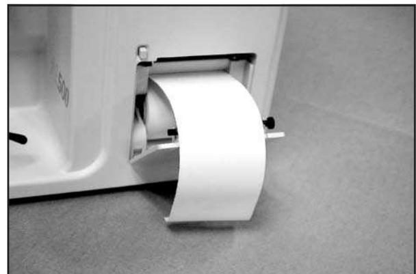
Figure 21. Lift Printer Cutter
