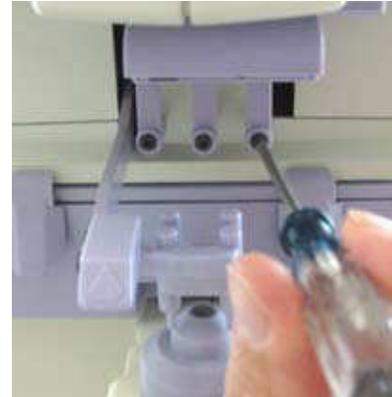
**Figure MM-4 Marking Pen Removal**
