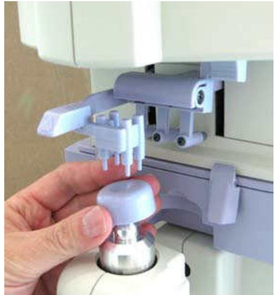
**Figure OP-18 Placing Contact Lens Cover**
