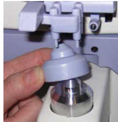
**Figure MM-6 Lens Stand Replacement**
