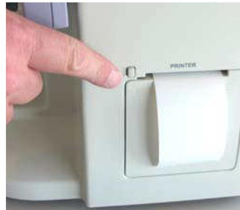
Figure MM-2 Door Release Button
