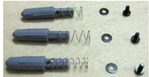
**Figure MM-5 Marking Pen Disassembly**
