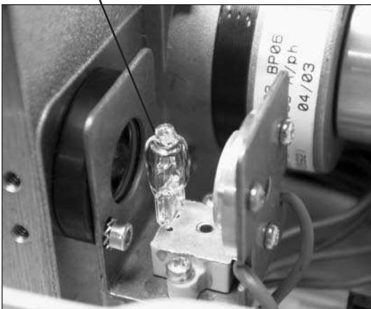
Figure 8 - Replacing the Halogen Bulb.
